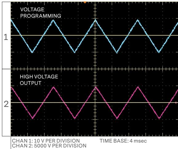
Figure C. 5HVA24-BP1 triangle wave input
