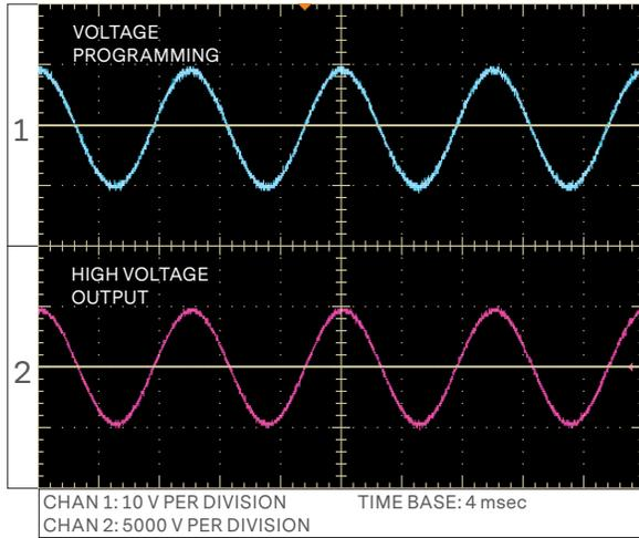
Figure A. 5HVA24-BP1 sine wave input
